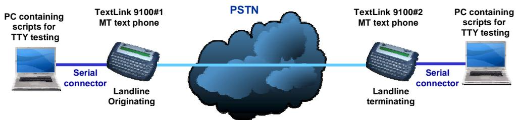
**Figure 6: Landline (PSTN)-to-Landline (PSTN) Field Test set-up using two TextLink 9100 MT's**
